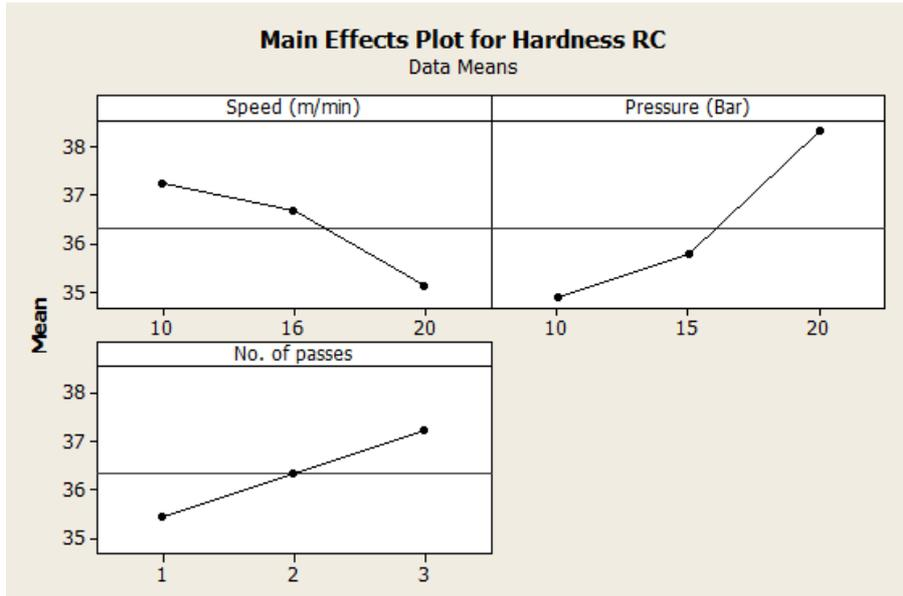
**Figure 5: Effect of Control Factor on Surface Hardness**
