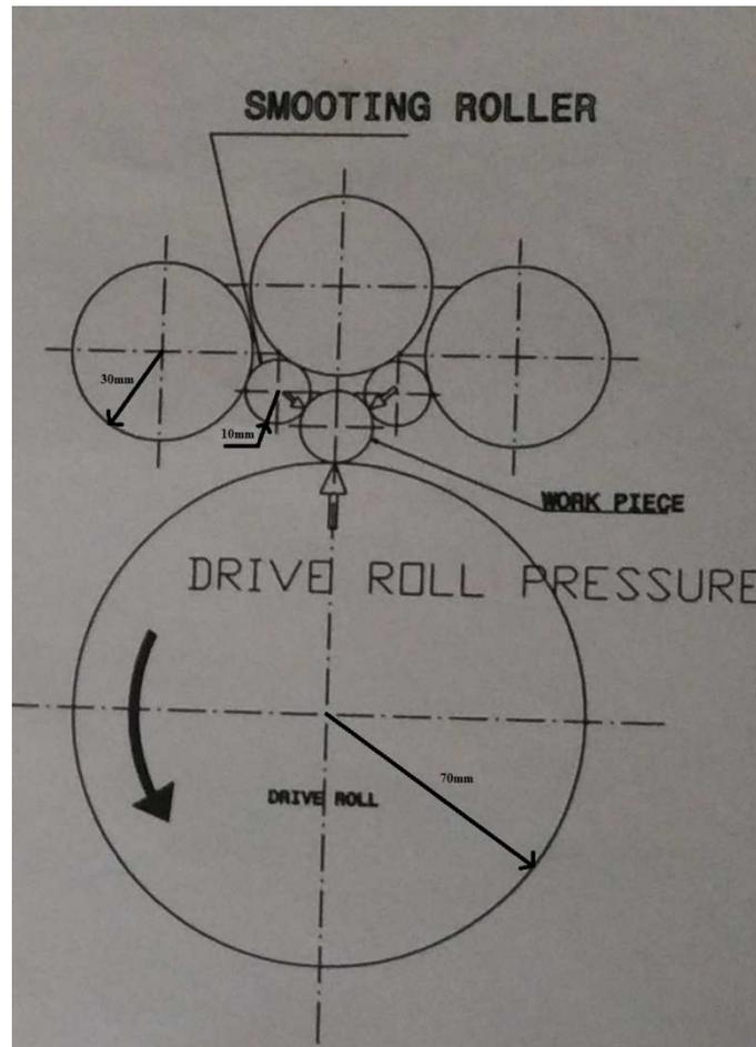
Figure 3: View of Multi Roller Burnishing Tool
