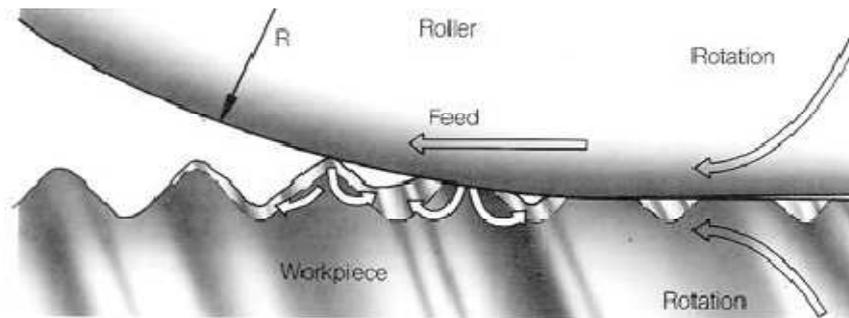
**Figure 1: Basic Operation of Burnishing**
